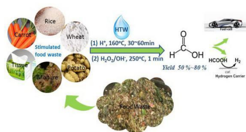
Figure 1. Proposed method for conversion of polysaccharide-rich food waste into formic acid.
